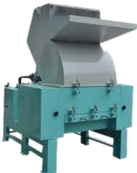
MACHINE 1 – ELECTRICAL CRUSHER (A)
